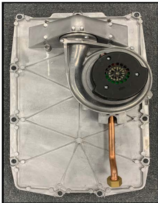
A typical front plate with fan assembly attached
