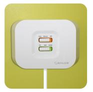
A constant orange light indicates that the receiver has lost RF signal and entered FAILSAFE MODE. In this event, your system will be switched on for 4 minutes, then off for 11 minutes. If you want to disable FAILSAFE MODE when RF link has been lost then move the slide switch on the receiver to either the manual or off position.
