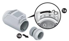
1. Separate the valve baseplate from the radiator controller. To do so, push the slide towards <sup>(2)</sup>.
