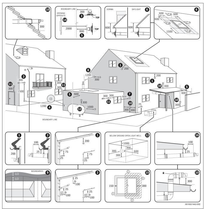
Fig. 27 Horizontal flue terminal positions
