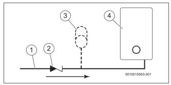
Fig. 9 Mini expansion vessel location
