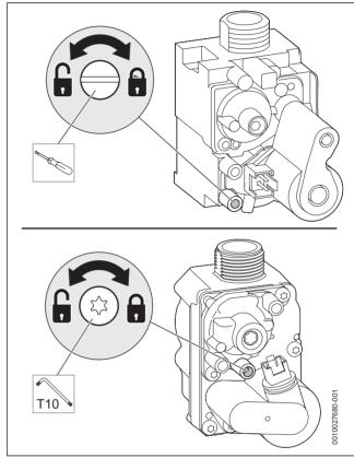
Fig. 54 Checking the gas supply pressure
