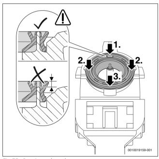
Fig. 75 Pressing on the gasket
