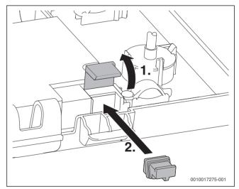
Fig. 91 Inserting the code plug
