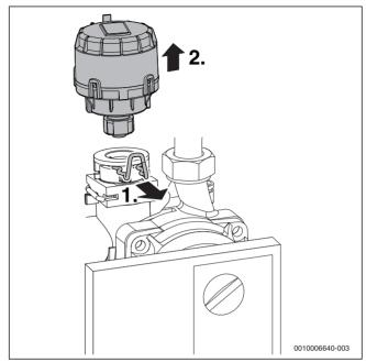
Fig. 87 Removing the motor of the diverter valve
