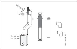
Fig. 22 Vertical flue option
