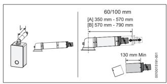
Fig. 13 Horizontal flue option
