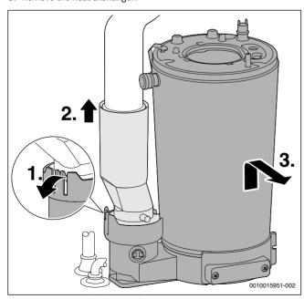
Fig. 89 Removing the heat exchanger
