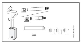
Fig. 20 Horizontal flue option
