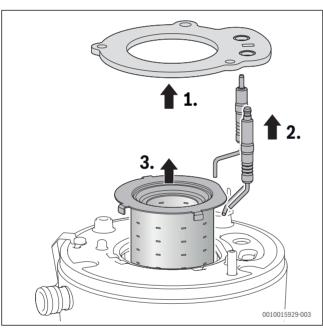
Fig. 65 Removing the burner
