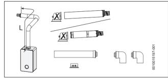
Fig. 19 Horizontal flue option
