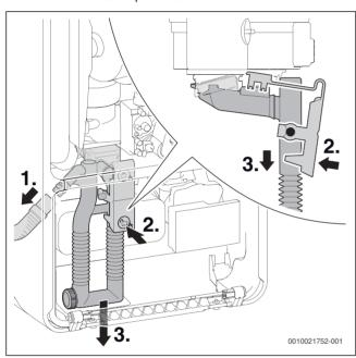
Fig. 71 Removing the condensate trap
