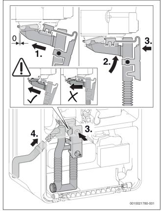
Fig. 76 Inserting the condensate trap
