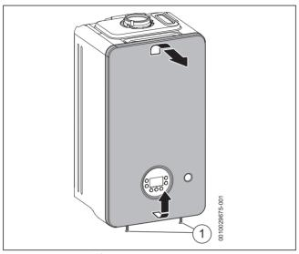
Fig. 78 Removing the front casing
