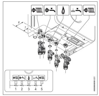
Fig. 38 Fitting the connection sets
