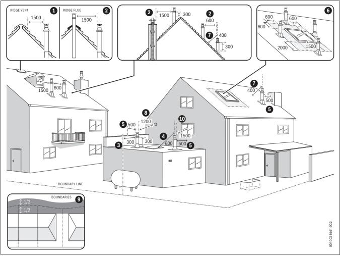
Fig. 26 Vertical flue terminal positions
