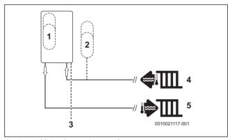
Fig. 4 Additional expansion vessel
