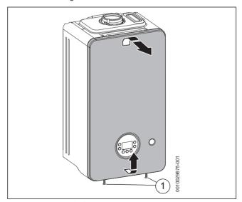
Fig. 40 Removing the front casing
