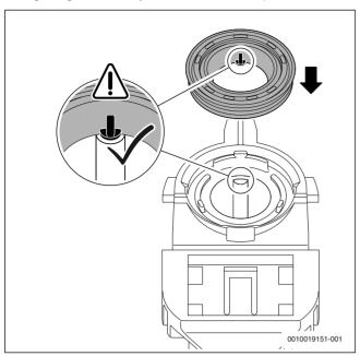
Fig. 74 Aligning the gasket with the condensate trap
