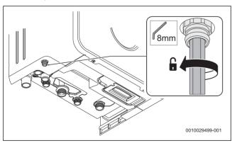
Fig. 79 Drain point
