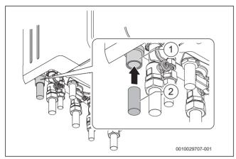
Fig. 42 Connecting to the condensate outlet connection
