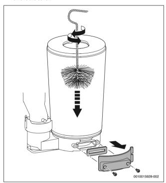
Fig. 68 Cleaning the heat exchanger
