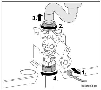
Fig. 83 Pull of the plug and undo the union nuts
