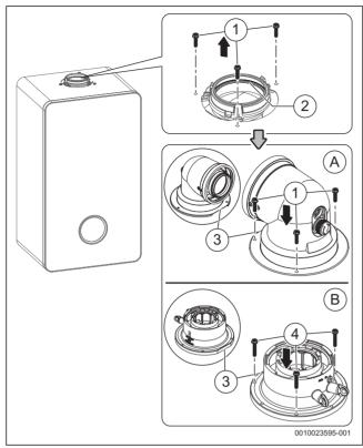
Fig. 45 Flue turret/adaptor connection
