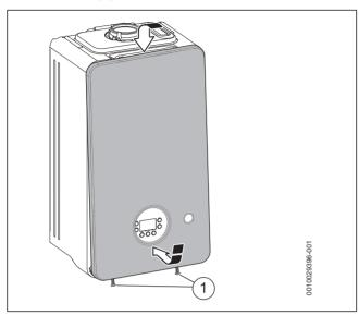
Fig. 59 Fitting the front panel
