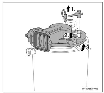
Fig. 63 Remove the burner cover
