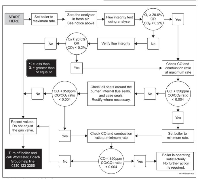
Fig. 56 Commissioning checks flow chart
