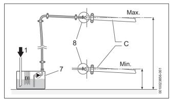
Fig. 31 Condensate pump example
