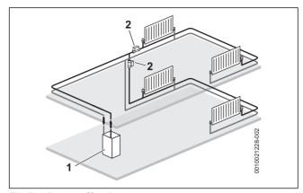
Fig. 7 Separated heating zones
