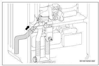
Fig. 39 Fitting the hose to the condensate trap
