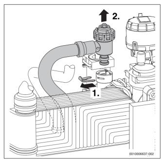
Fig. 80 Remove the pressure relief valve (heating circuit)
