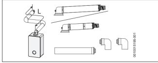
Fig. 17 Horizontal flue option
