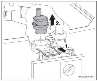
Fig. 86 Removing the automatic air vent valve
