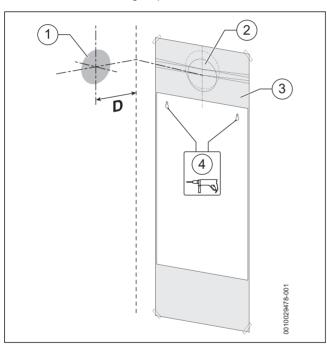
Fig. 37 Wall mounting template
