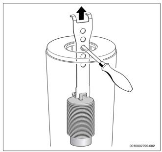
Fig. 67 Removing the bottom baffle
