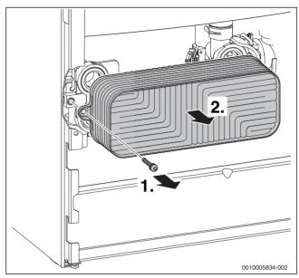
Fig. 82 Removing the plate heat exchanger
