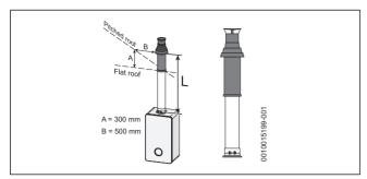
Fig. 21 Vertical flue option
