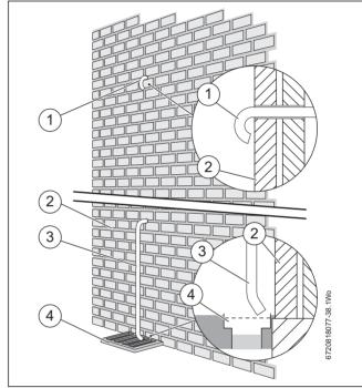
Fig. 36 Pressure relief pipe work
