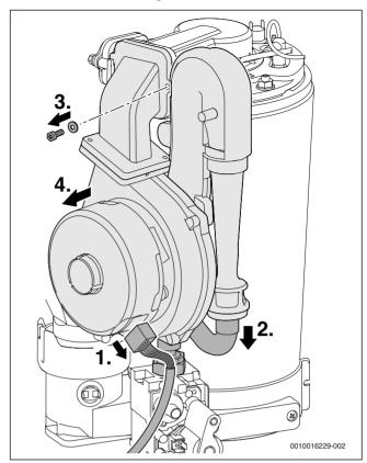
Fig. 62 Removing the fan with mixing device
