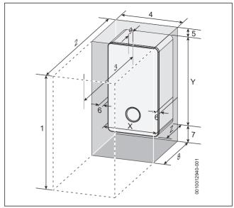
Fig. 11 Appliance minimum clearances
