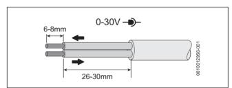
Fig. 49 Low voltage (signal cables) preparation
