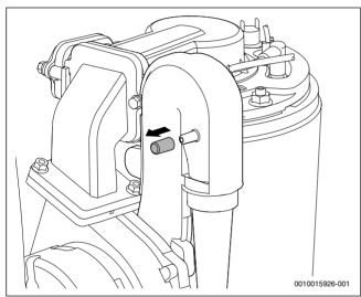
Fig. 61 Test nipple at the mixing device
