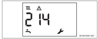
Fig. 93 Example: non-blocking fault
