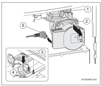
Fig. 85 Removing the pump
