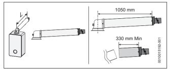
Fig. 14 Horizontal flue option
