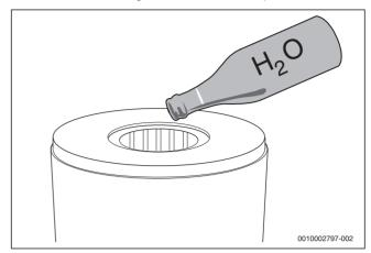
Fig. 70 Purge the heat exchanger with water
