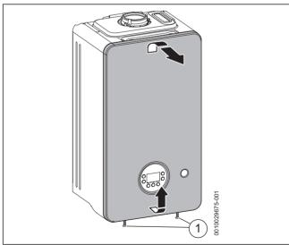
Fig. 60 Removing the front casing
