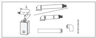
Fig. 16 Horizontal flue option
