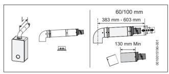
Fig. 12 Horizontal flue option
