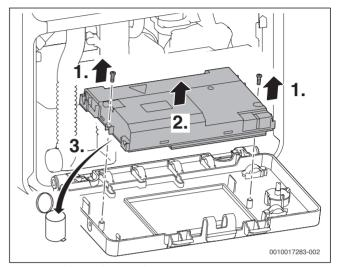
Fig. 90 Replacing the control unit
