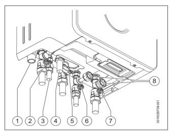
Fig. 41 Connections on the gas and water side
