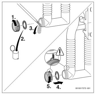
Fig. 72 Cleaning the condensate trap
