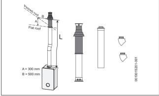
Fig. 23 Vertical flue option
