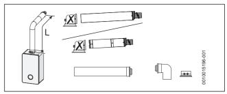
Fig. 18 Horizontal flue option
