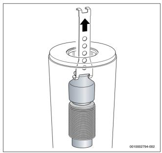
Fig. 66 Remove the top baffle
